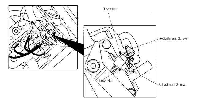
Adjust HIGH IDLE: First make sure there is NOT a load on the machine. Use the 10mm wrench to loosen the lock nut. See Figure F.9 for location of adjustment screw and lock nut. With the 10mm wrench turn the adjustment screw counterclockwise to increase the high idle RPM. Note: It is usually NOT necessary to cut or remove the wire and seal. Adjust the speed until the tach reads between 3650 and 3700 RPM.
